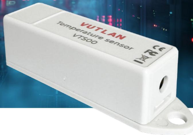
**VT500** Temperature sensor is an analog plug-and-play temperature sensor for indoor use only. Can be connected to any of the analog ports (A1...A8) of Vutlan monitoring systems. The accuracy of the sensor is  $\pm 0.15$  °C at room temperature. The maximum distance from the monitoring unit (or sensor extension unit) is 100 meters.
