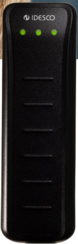
Highly secure, open technology MIFARE DESFire reader in a range of housings and keypads up to moisture, dust, and vandal proof, compatible with other manufacturers' DESFire devices. The reader is used together with VT485r OSDPv2 reader extension slot
