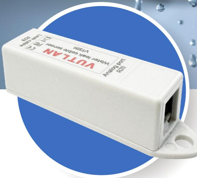
The **VT591 Water Leak Sensor** is designed to detect water leaks by sensing a drop in resistance along the connected WLC Water Leak Cable. This sensor requires the use of a WLC Leak Cable, which is ordered separately and available in various lengths to suit different installation needs.
