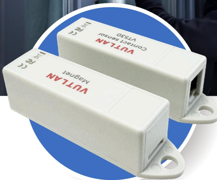
The **VT530 Access Sensor** is essential for access control and is designed to monitor the status of doors and windows (open or closed). It consists of two parts: a magnet and a sensor, ensuring accurate detection of access points being opened or closed. It can be connected to any analog port (A1...A8) of the Vutlan monitoring unit and supports daisy chaining, allowing multiple sensors to be linked in a series for easy and scalable installations.
