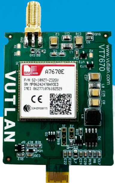
Allows to receive and send SMS and provides network reservation: e.g. if the LAN connection fails, the Ethernet connection is secured using 4G.
