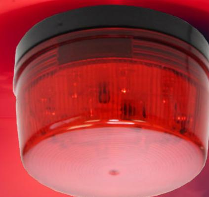
The **VT105 LED strobe light** is a 12V DC device designed to provide flashing light alerts for warnings and alarms. It connects to the 12V DC, 0.25A electronic relay output of Vutlan monitoring systems, offering a visual notification in case of triggered alarm events.
