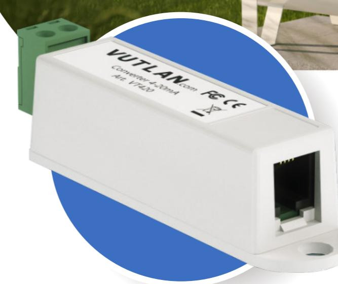
The **VT420** is a converter of direct current 4-20mA used for measurement of constant current on 4-20mA from different 3rd party sensors and converting data into the format of the Vutlan monitoring system. The system interface allows you to assign the sensor and introduce the function data conversion.
