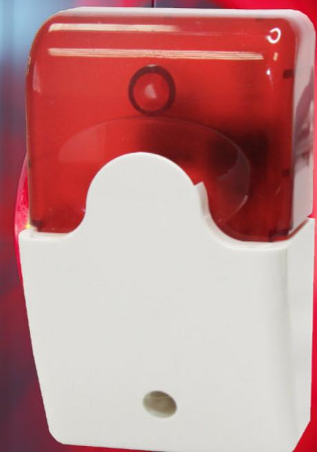
The **VT103** is designed for light and sound alarms in monitoring systems. It can be connected to a 12V DC, 0.25A electronic relay output of Vutlan monitoring systems to provide a visual or audible alert when an alarm event is triggered. This makes it ideal for scenarios where immediate local alerts are needed to inform users of system issues.
